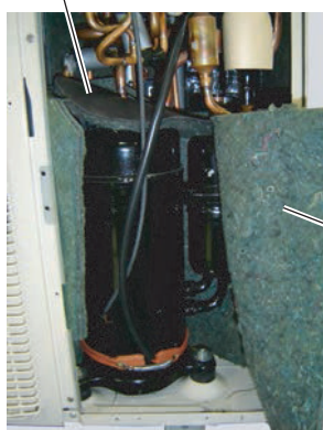
Remove the COMPRESSOR COVER A and TOP.
