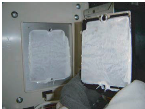
Spread the heat transfer compound on ACTPM when you exchange ACTPM by the repair.
