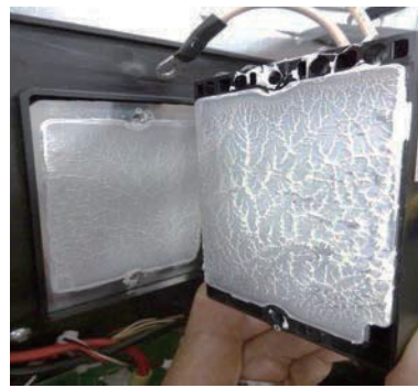
Spread the heat transfer compound on ACTPM when you exchange ACTPM by the repair.
