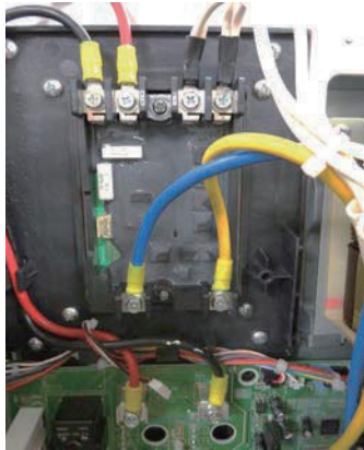
Remove the screws and lead wires.
